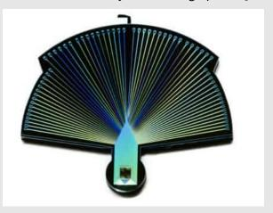
Figure 3.6: Close-up photograph of the PEACOQ detector which can detect photons at a rate of a gigahertz. 128
