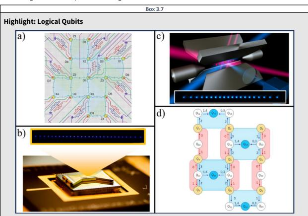
Figure 3.7: a) False-color image of the superconducting-qubit device realizing the surface-17 code; <sup>136</sup> b) an ion trap used to demonstrate a Bacon-Shor code (array of ytterbium ions inset); <sup>137</sup> c) illustration of the ion trap used to demonstrate the color code (array of calcium ions inset); <sup>138</sup> and d) mapping of heavy-hexagon code onto 23 transmon qubits. <sup>139</sup>
