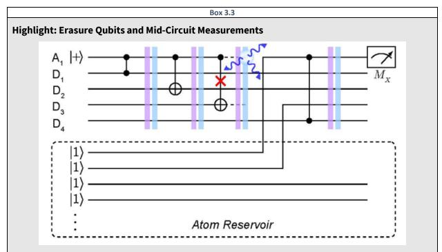
Figure 3.3: Schematic quantum circuit with programmed replacement of qubits with erasure errors, based on mid-circuit measurements, capable of detecting leakage from the computational subspace. 48
