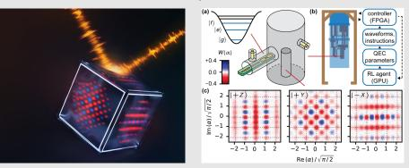
Figure 3.4: (Left) Representation of a logical qubit embedded into the state space of a harmonic oscillator using grid code, represented here by the faces of a cube.<sup>93</sup> Quantum error correction protects these grid states from corruption by a noisy environment, symbolized by the ray. (Right) Description the experimental system and quantum states involved in error correction.<sup>94</sup>
