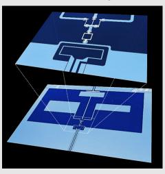
Figure 3.2: The central working region of a new superconducting quantum computing device. In the lower section, the three large rectangles (light blue) represent two qubits, at right and left, with a readout resonator in the center. In the upper, magnified section, a microwave antenna (large dark-blue rectangle at bottom) is used to induce a magnetic field in a SQUID loop (smaller white square at center), which activates the toggle switch. <sup>28</sup>
