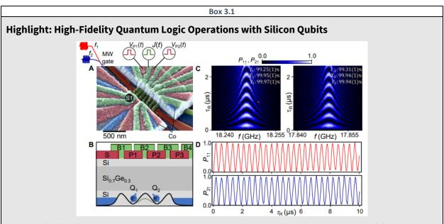
Figure 3.1. (Left) Quantum dots trapping electron spin qubits in a silicon-germanium heterostructure. (Right) Observation of spin qubit operations.<sup>14</sup>
