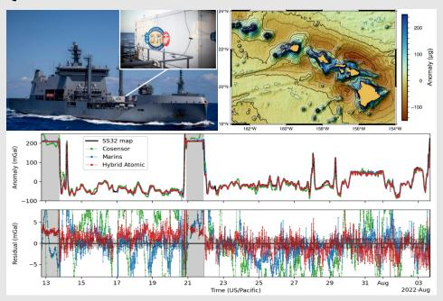
Figure 3.5: (Top left) The HMNZS Actearoa underway at RIMPAC with an ONR shipping container used to support the various experiments is visible on the deck.<sup>122</sup> (Top Right) Gravity map around Hawaii used for gravity map matching. (Bottom) Measurements of the RIMPAC data showing micro-g deviation of the atomic gravimeter verses other gravity anomaly map. <sup>123</sup>
