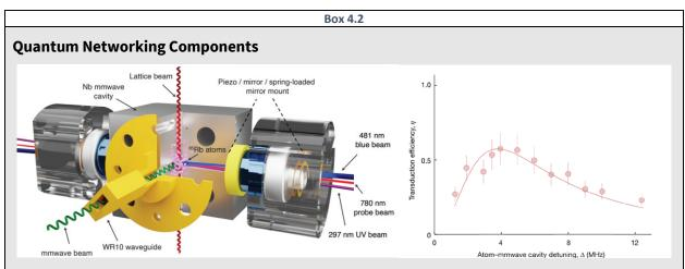
Figure 4.3: (Left) Apparatus for microwave to optical photon transduction with atoms trapped in crossed superconducting and optical cavities. (Right) Experimental data on transduction efficiency. 146
