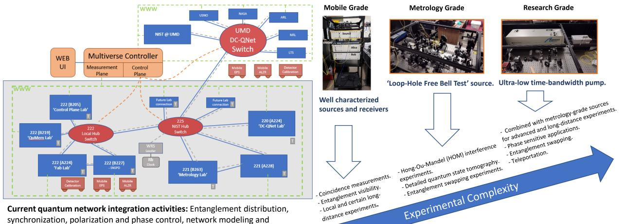
**Current quantum network integration activities:** Entanglement distribution, synchronization, polarization and phase control, network modeling and management, quantum/classical coexistence, metrology nodes for link characterization, component testing etc.
