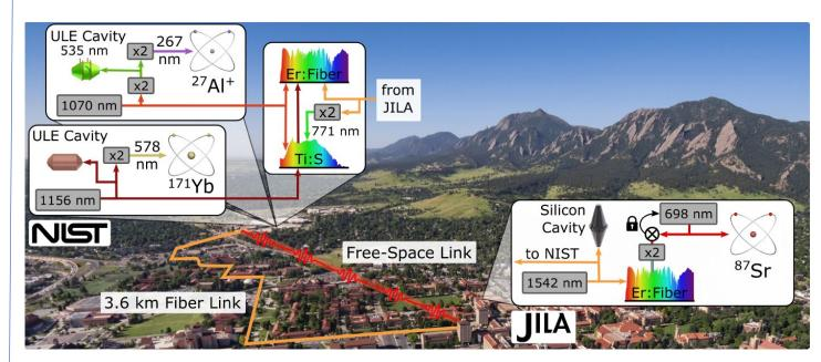
Comparing optical lattice clocks and trapped ion clock using frequency combs and optical networks (fiber and free-space)
